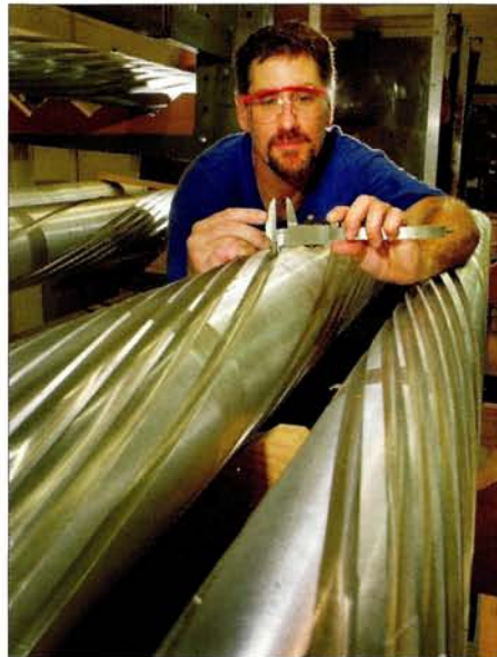
In a spin: the corkscrew design of RHIC's Siberian snake magnets causes the magnetic field to spiral along the direction of the beam. (Brookhaven National Laboratory.)
